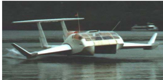
The Hoverwing HW2VT scale prototype of 80 seat ferry by Fischer Flugmechanik
