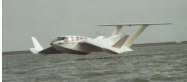
The AF8/SF8 built by Fischer Flugmechanik and AFD (Germany) for Flightship Ground Effect (Australia) 2001.
