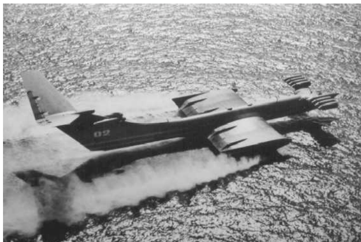
Figure 2: The KM ‘Caspian Sea Monster’ – Russian 550 tonne Ekranoplan of 1966.
