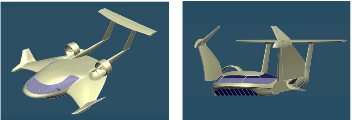
Figure 4. HW-20 showing blended/lifting body and wings folded
