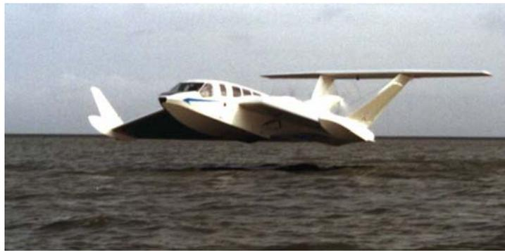
Figure 3: Airfish 8/Flightship 8, eight passenger vessel launched in 2001
