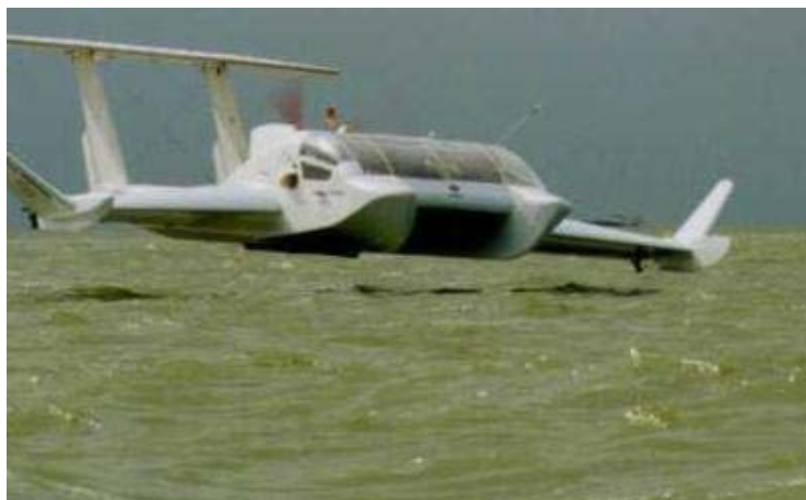
Figure 7: The HW2VT 2 seat technical demonstrator in 1997. This was a scale model of an 80 seat concept.
