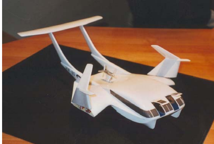
Figure 6: The HW-80 showing the blended/lifting body/hull and folding wings
