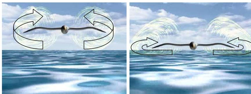
Figure 2. WIG = Distortion of airflow around a wing due to the presence of a surface
