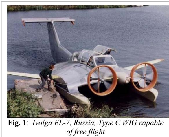
**Fig. 1:** *Ivolga EL-7, Russia, Type C WIG capable of free flight*
