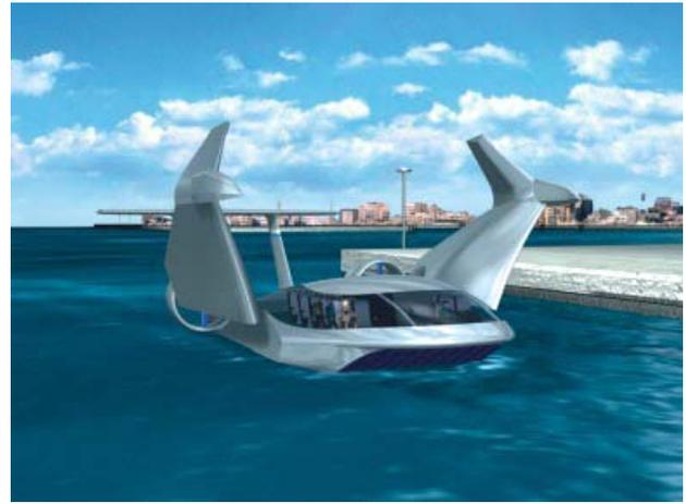
**Fig. 8:** HW-20 concept showing blended/lifting body and wings folded. \*
