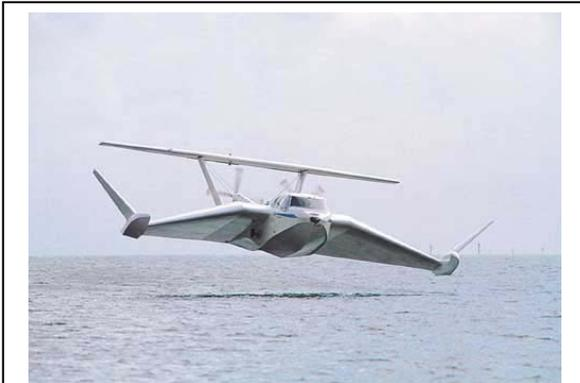
**Fig 4:** First-generation Airfish 8/Flightship 8, eight passenger vessel launched in 2001
