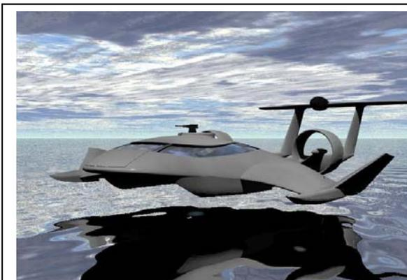
**Fig. 11:** *The HoverWing HW20 100 knot concept. Accommodates 12 fully armed troops, or two quad bikes and other equipment. Armed with 50 cal chain gun with remote/stabilised gun laying for littoral patrol/special operations.\**
