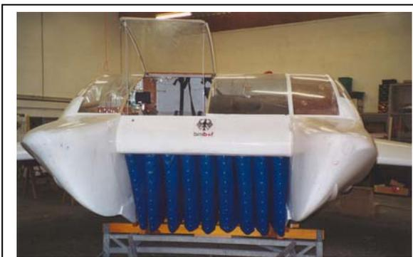
**Fig. 5:** Bow of HW2VT showing retractable skirt
